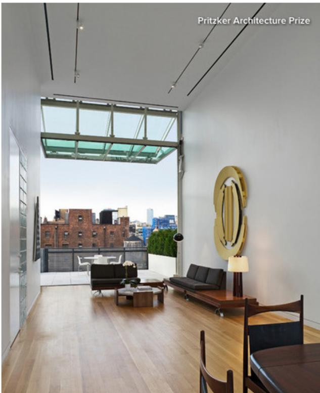
This upward-pivoting 20-foot-tall sectional door opens this entire penthouse apartment to the city and offers proof that, when carefully designed, the overhead door can work in almost any climate, even one as extreme as New York's. The pivoting panels create a folded, glazed roof for the outdoor area.
