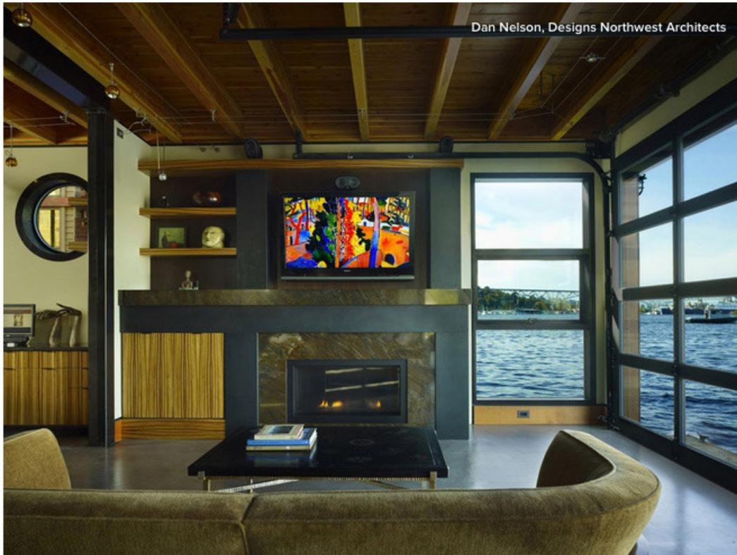
The track and mounting hardware here have been treated very intentionally and made a part of a family of design details in which black has been designated for use on all hardware. The unification of design elements is a great trick for leveling up the refinement of a utilitarian assembly.
